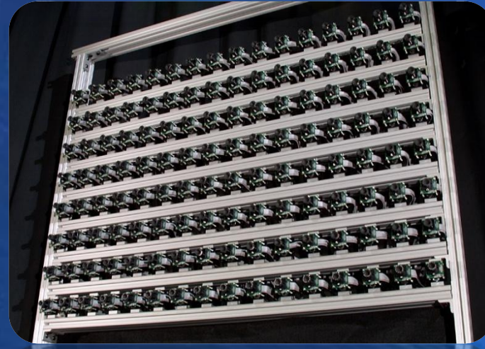
The Stanford multi-camera system
