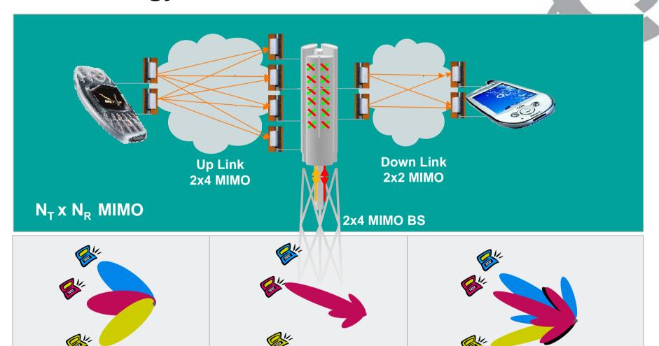
**Fixed beam:** Users served by nearest fixed beam. Beams generated from antenna columns. Example has 3 way SDMA. (AABS has beams but no SDMA)
